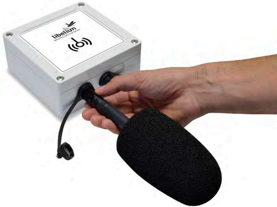
Figure: Connecting the sensor probe to the enclosure
