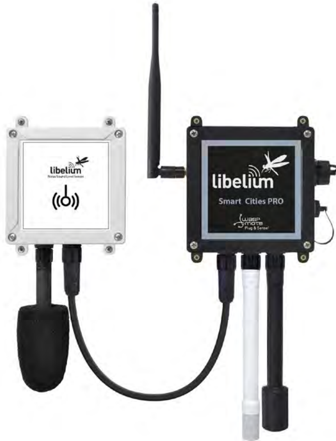
Figure: Connecting the data cable to the associated Plug & Sense! Smart Cities device
