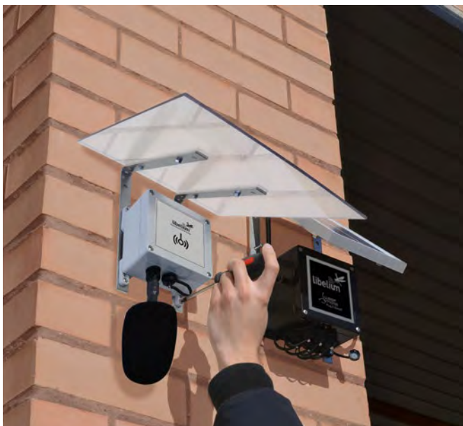
Figure: Installing the Noise Level Sensor on a wall
