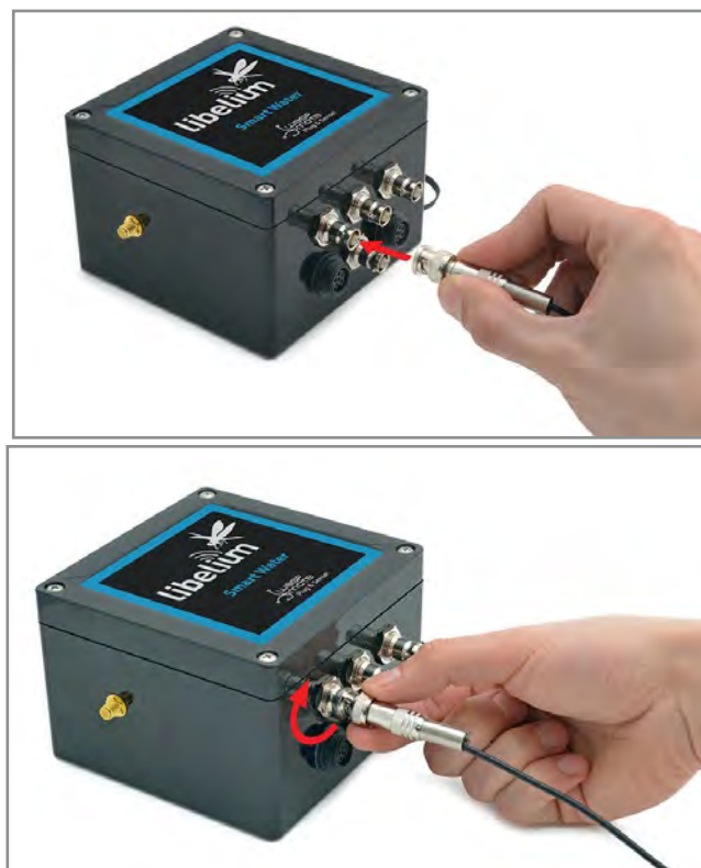
Figure: Images of the procedure to change the probes for the Smart Water Plug&Sense!
