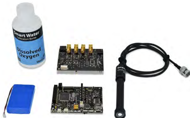
Figure: Image of the material necessary for the dissolved oxygen calibration process
