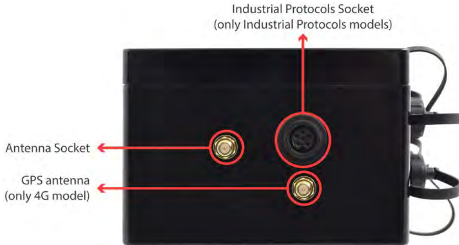
Figure: Antenna side of the enclosure
