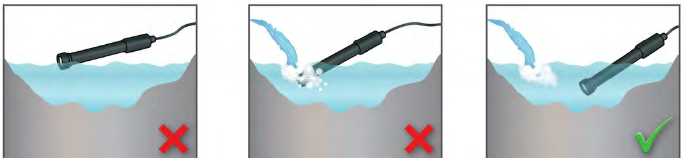
Figure: Image of several situations with the sensor incorrectly installed
