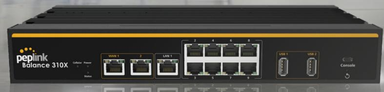
The Balance 310X has a fanless design and a wide temperature range. Drop it into demanding environments and run it for years without worry.
